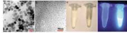
Fig. 2 (a) TEM image of CoFe 2 O 4 nanoparticles, (b) TEM image of GQDs, (c) Bright field optical image and (d) 365nm UV light optical image of GQDs (right) and blank solvent (left).
